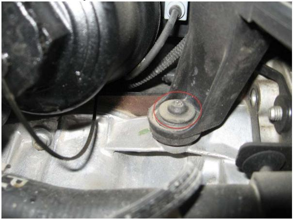
Carefully remove the pipe from the car them remove the 2 remaining clamps using a 7mm for the worm clamp and channel locks to remove the noise pipe clamp. We will drill the hole here:
