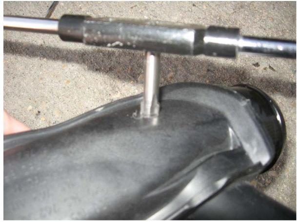
Follow the instructions inside the DO manual to properly assemble the nozzle and check valve. Once completed carefully thread the nozzle into the throttle pipe:
