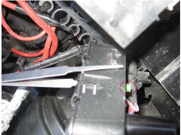
Add silicone to the wire to ensure everything is water tight and insert from the bottom side. VW wanted this panel to stay water tight so once I had the wire in there I double checked that the new wire was indeed water tight. Once completed push the pink clip (2 pictures back) back to its original position:
