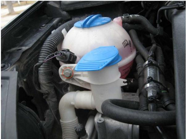
**Step 3, Install washer adapter:** Drill a hole using the 7/8 drill bit into the tank::
