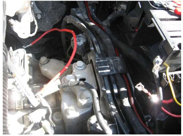
Solder the black power wire to the yellow repair wire we installed earlier:
