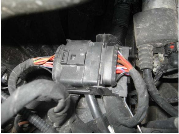
Strip wire, attach green wire from the DO controller, and then solder together. The wire is the Lilac/Green wire in pin 14:
