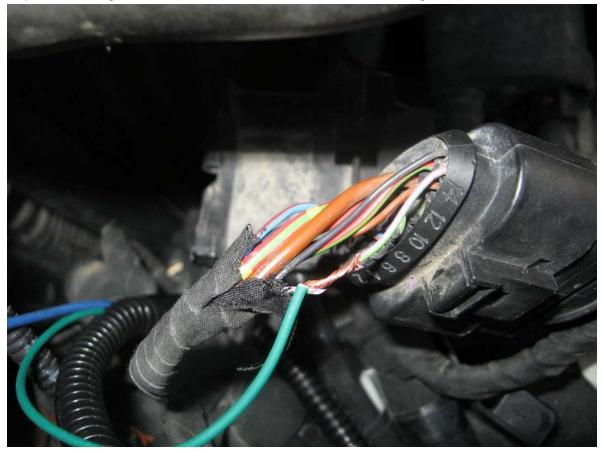
The wiring in the engine compartment is now complete. The blue wire pictured below will be run to the pump in stage 2:
