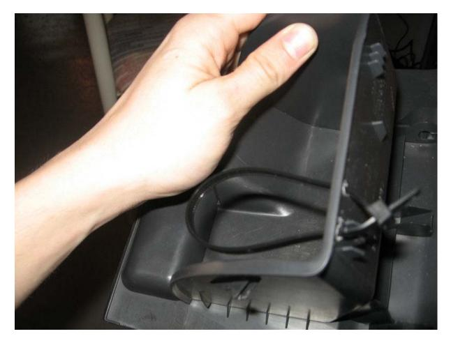
Secure the relay to the existing wiring above the black cover using electrical tape, re-install the black cover, the cubby tray and this stage is complete.
