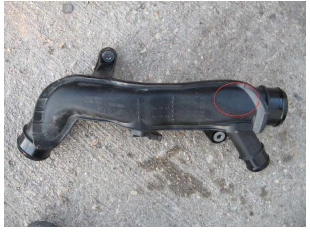
**Step 2, Install nozzle:** Drill the hole with an 11/32 drill bit,then tap using a 1/8<sup>th</sup> NPT tap:
