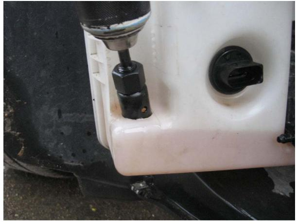
Insert the adapter and tighten with fingers:
