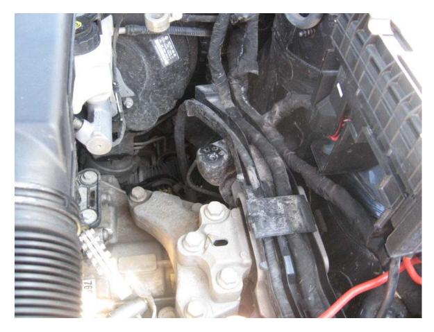
Step 3, Remove relay panel: First remove the positive wires from the relay panel. You will need a 10mm socket (red) and an 8mm socket (blue):
