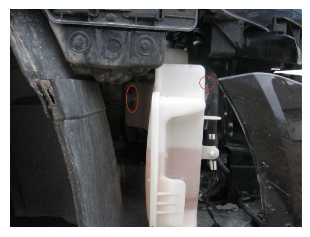
Remove the top bolt (red) holding the filler spout to the frame then remove the tank from the car:
