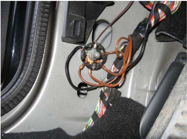
Remove a section of insulation from the ground wire going to the controller and splice in the black side from the relay:
