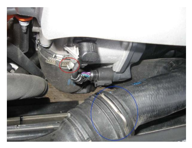
Use an 8mm socket to remove the top bolt of the pipe (red) and a 7mm socket to remove the lower clamp (green). Disconnect the MAP sensor (blue), Note the clip is behind the hose in this picture
