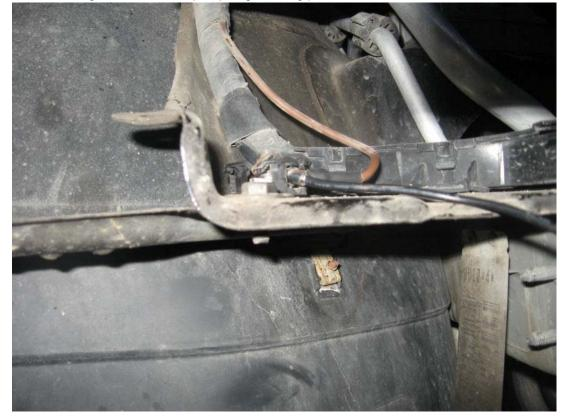
Run the blue wire that was left over from stage 1 down from the connector where we attached the green wire near the driver side horn, then in front of the radiator alongside the passenger fog light loom. Attach it to the positive side of the pump:
